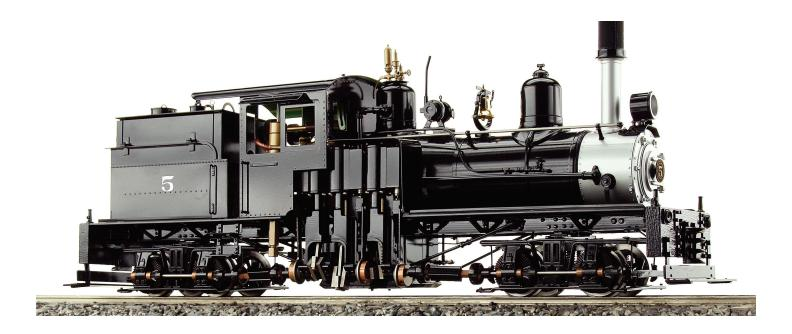
Shay locomotives were developed by Ephraim Shay. His first successful engine that we would recognize today as a Shay locomotive was produced in 1880 by Lima Machine Works (later, Lima Locomotive Works), who would go on to produce approximately 2,700 up until 1945, when production ceased.
